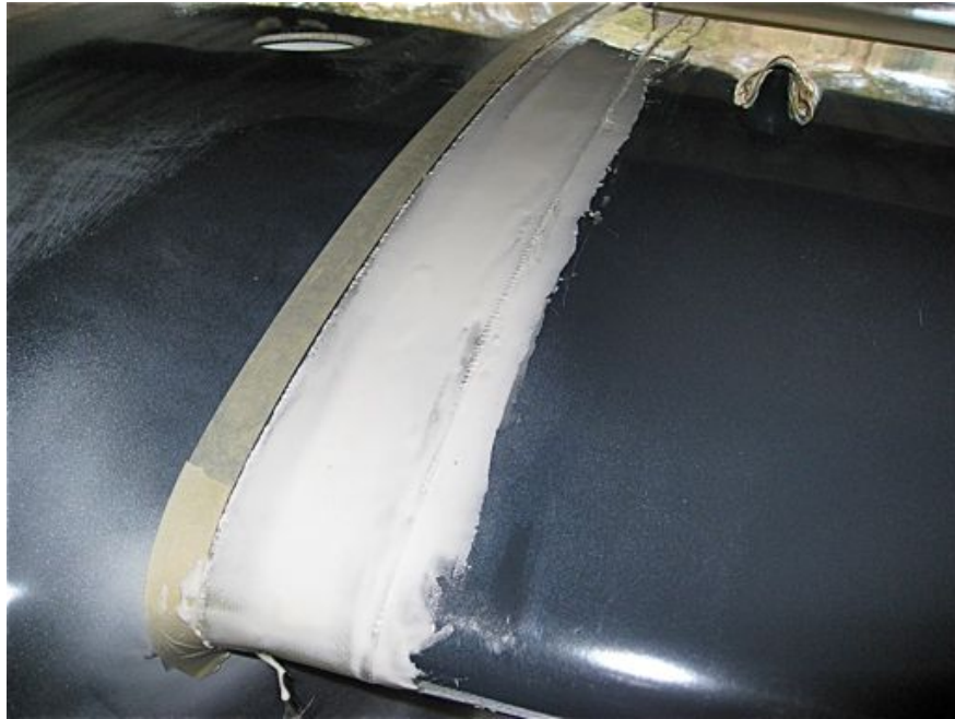
While outside, the wing to fuselage fairings were laid up, as shown on pic #188.
