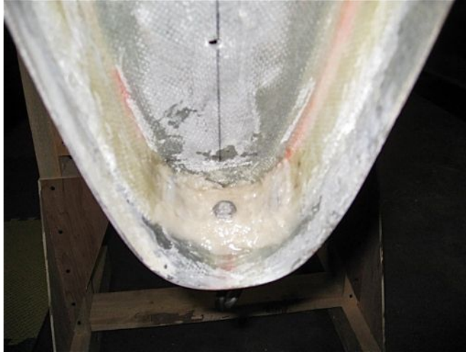
Pics # 197 and #201 show the tail down eye bolt and aluminum plate. A 5/6" nut was attached with JB Weld to the plate and then it was cotton floxed and glassed onto the inside of the bottom fuselage, behind the rudder post.
