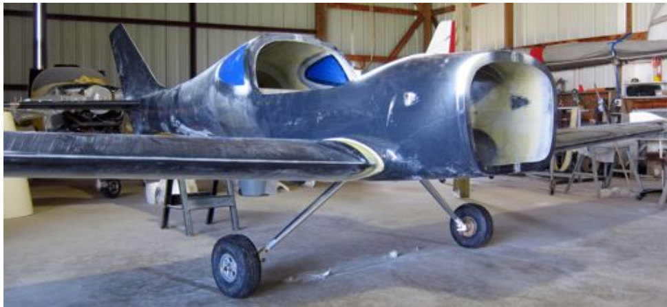
On the mains after installing and setting toe (week 1)
