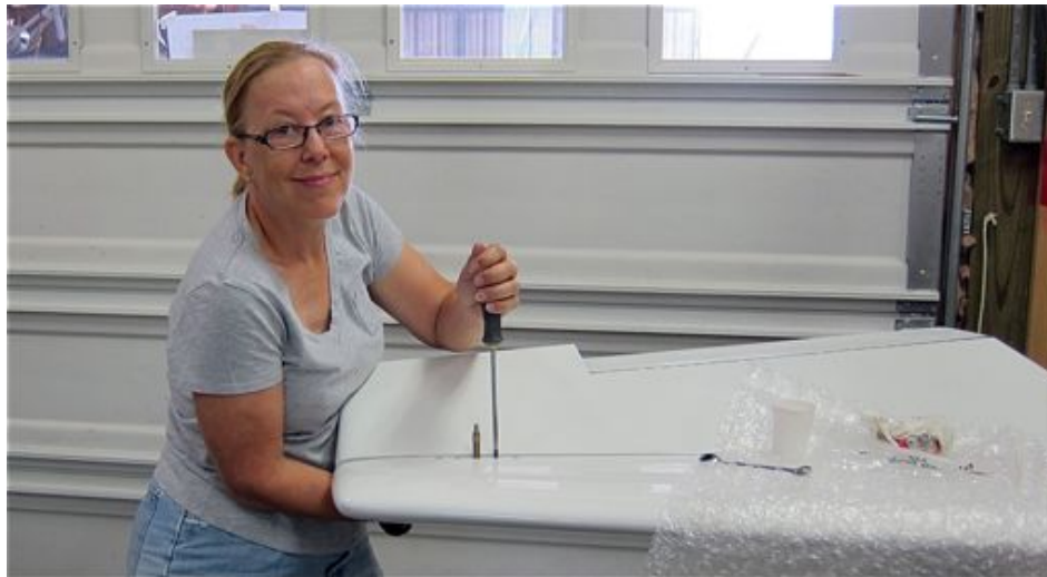
Donna installing the elevators (week 2)
