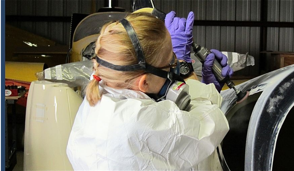
Donna sanding the gel coat to install the opera windows (week 1)
